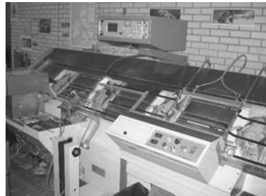
The recently acquired high speed collator (left) and Rilecart wiro binding machine (right)
